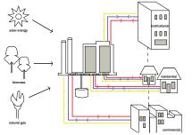
(Above) Diagram showing the inputs into the power plant and the outputs of electricity, steam and chilled water. (Right) A rendering of the potential of the power plant to be retrofitted with solar panels and green walls to increase energy efficiency.
