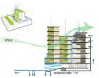
Collect rainwater from the roof and collect gray water from community to the garden and recycled water treatment system.
