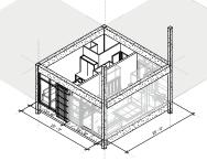
Utilizing a hybrid prefabrication method, each individual residence is composed of a kitchen and bathroom pod and adjustable partition panels. A raised access floor system enhances flexibility and facilitates the installation of partition panels. Hollow core slab sections support the floor and roof. A green roof system adds much needed permeable surface to the area and aids in water retention during heavy rains, thereby easing the load
