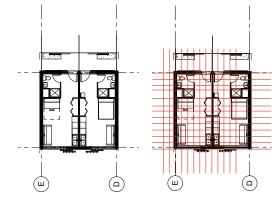
The tartan grid frame breaks down further into a 2' x 2' interior grid within each unit. Movable sections of wall panels allow the occupant to customize their interior as needed, or join multiple units together. The raised access floor facilitates the relocation of plumbing and electrical lines, allowing greater design possibilities as functional needs change or equipment becomes outdated.
