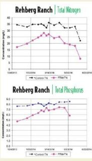
The Rehberg Floating Treatment Wetland (FTW) has proven effective at removing nitrogen and phosphorus.
