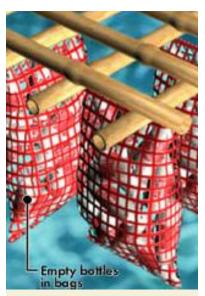
Plastic bottles in mesh bags are connected to a bamboo frame, supporting the island and allowing it to float.
